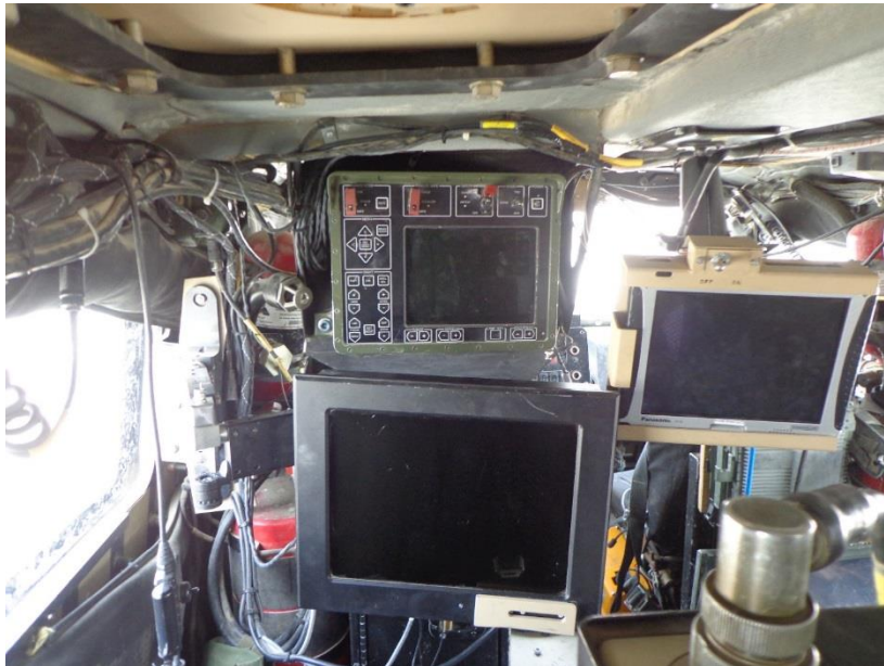
Current crew station includes separate displays for each of the enablers in use, limiting room for future capability growth and creating integration challenges
