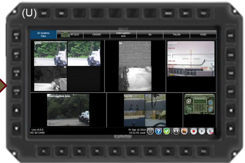
MVD combines enablers onto single display for simultaneous view and control of all enablers at every crew station
